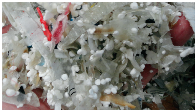
Fiber-free rejects including troublesome styrofoam and plastics
