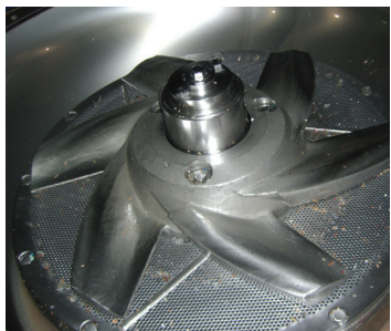
Float Purger rotor and bed plate
