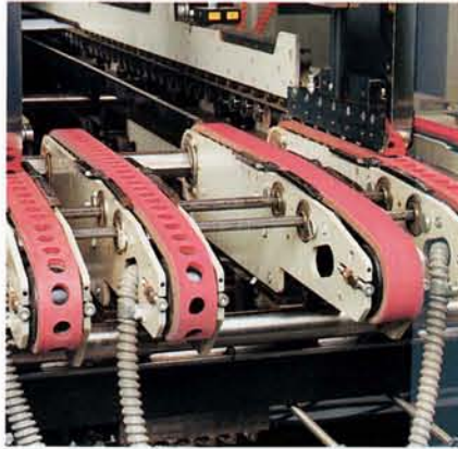
Vacuum-assisted timed belt feeder for problem-free feeding.
