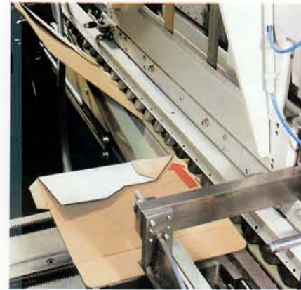
Wheel-type calibrating units calibrate the cartons in cross direction ...
