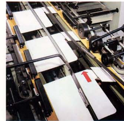
... and calibrating belts ensure precision folding.
