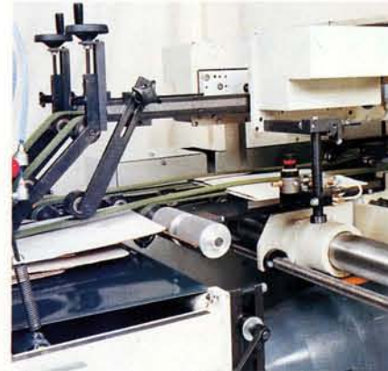
Short set-up times with the motorized setting of the transfer station.
